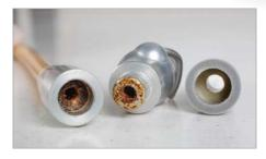
A used metal SE valve, rubber cup and SE tailpiece connected to the suction line
