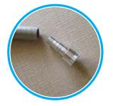
Push the new DOVE® tailpiece on the existing vacuum tubing, using dish soap or natural lubricant as needed.
