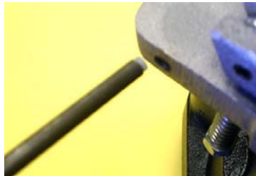
In the unlikely event the locking pin should come out of the hole, simply re-insert with the white plastic tip facing inward toward the post.
